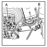
A. Remote Negative B. Positive Terminal After unsnapping and opening the black cap on the positive (+) terminal on the top of the battery, clamp the jumper cable to the terminal.
